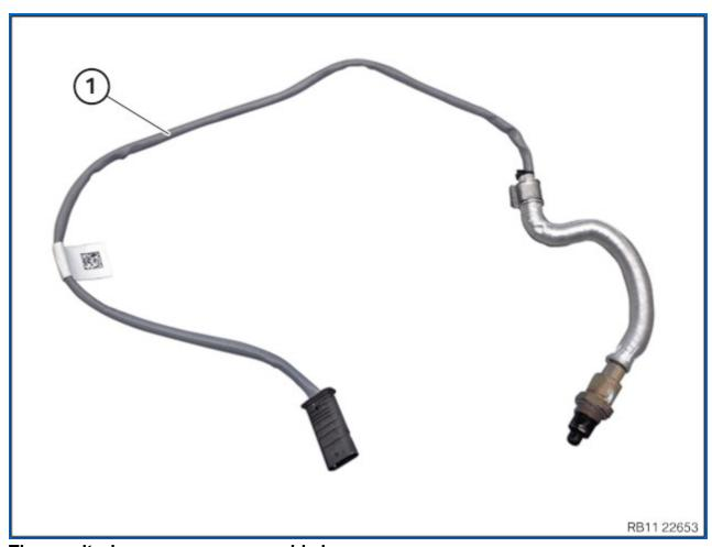
The monitoring oxygen sensor cable is grey (1).
