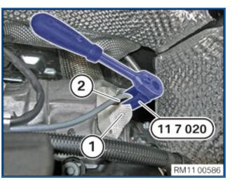
Slightly bend up heat protection film (1). Remove monitoring oxygen sensor (2) with specia 11 7 020.
