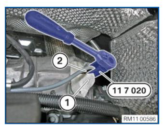
Screw in monitoring oxygen sensor (2) and tighten tool 11 7 020.
