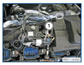
Connect monitoring oxygen sensor connector (1) a holder.
