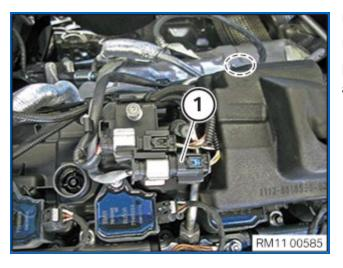
Unclip monitoring oxygen sensor connector (1) fro Unlock and disconnect monitoring oxygen sensor Detach monitoring oxygen sensor cable from the harea marked.
