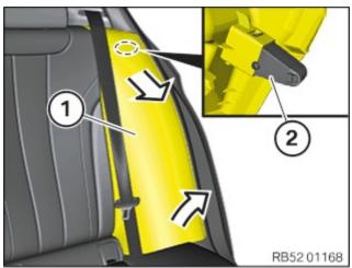
Reach behind the backrest side section (1) from the top and unclip the backrest side section (1) from the latch mechanism (2) to the front.
