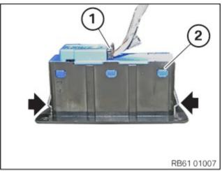
Unlock and disconnect the connector (1) on the switch (2).
