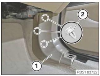
Loosen the side trim panel (1) at the clips (2) and remove it toward the inside.
