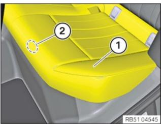
Release rear seat (1) in area (2) in upward direction from the latch mechanisms.
