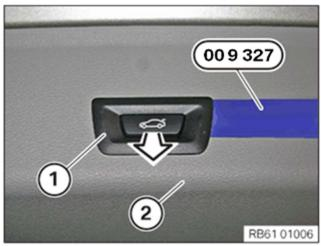
Lever the switch for the tailgate lift (1) out of the tailgate trim panel (2) with the special tool **0 496 571 (00 9 327)**.
