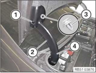
Loosen expanding rivet (1).
