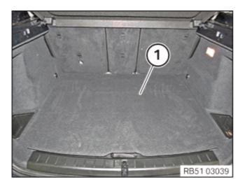
Attach luggage compartment floor trim panel (1) at front in guides and lay down at rear.
