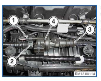
Unlock connector (1) and remove. Unlock tank ventilation line (2) and disconnect. Unlock tank ventilation line (3) on throttle body and disconnect. Detach tank vent valve (4) from holder and remove.
