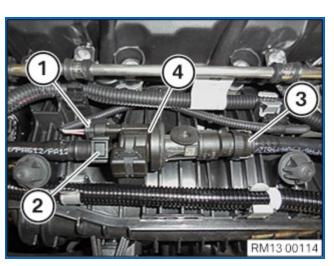
Attach connector (1). Connector (1) must engage audibly. Plug in tank ventilation line (2). Tank ventilation line (2) must snap audibly into place. Connect tank ventilation line (3). Tank ventilation line (3) must snap audibly into place. Fasten tank venting valve (4) to the holder.
