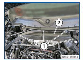
Release screws (1). Feed out cover (2) and remove.
