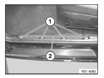
If necessary lift clip (1) from floor panel (2) and clip on door sill cover strip.
