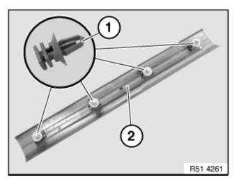
*Installation note:* Replace defective clips (1) on door sill cover strip (2).
