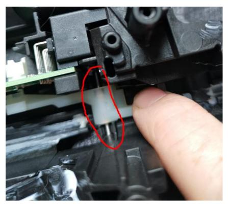
With this out, you will be able to see if the torsion spring is broken – mine clearly was. I carefully removed the spring and stretched it out 1 full revolution. It will need to be **past** 180degrees to push the white lever up.
