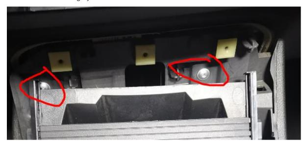
From the rear seats, pull up on the whole centre island, and it should pop up and pull out. Make sure you have not missed any cables, plugs or sensors attached to the centre island. It is a bit heavy, lift carefully over the gear selector and out the vehicle.
