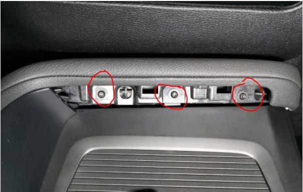
Remove trim and expose 2 hex screws on the passenger side of centre console. Remove both screws (Hex20) This can be done with the passenger seat in the car. (Put seat all the way back, and in lowest sitting position)
