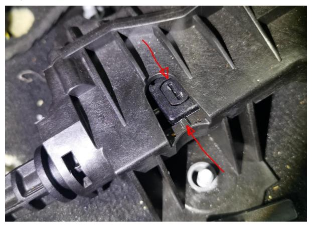
Once lined up, you need to lift the whole assembly, and rotate anti-clockwise so you can see the underside.
