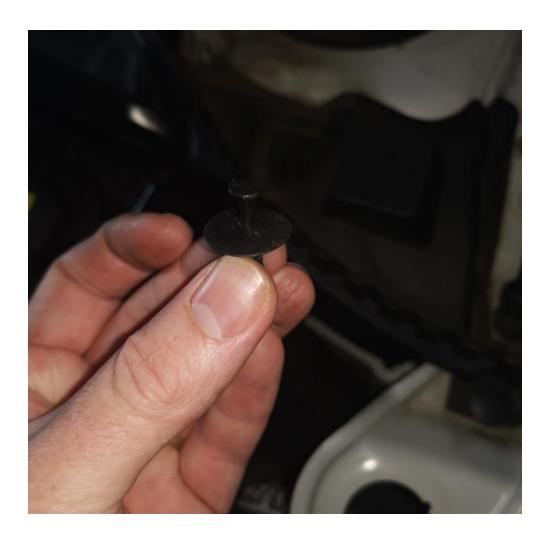
The leaf guard can pull up and out of place. This will expose the negative terminal of the battery which is all you need to disconnect. Size 10 socket.
