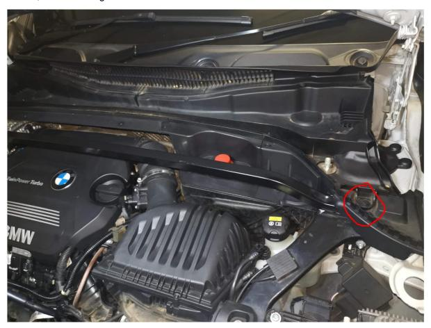
Remember to pull out the centre pin with a screwdriver or trim-tool BEFORE trying to pull the whole clip out:
