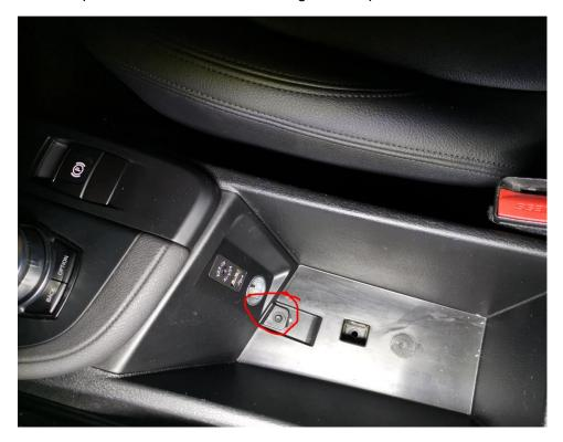
Use plastic trim tool, to pull forward the face plate with USB, Lighter socket and Audio. There are 2 clips at the top that will pop off.
