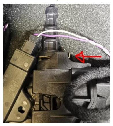
Remove all 4 size 10 bolts holding down the gear selector unit.
