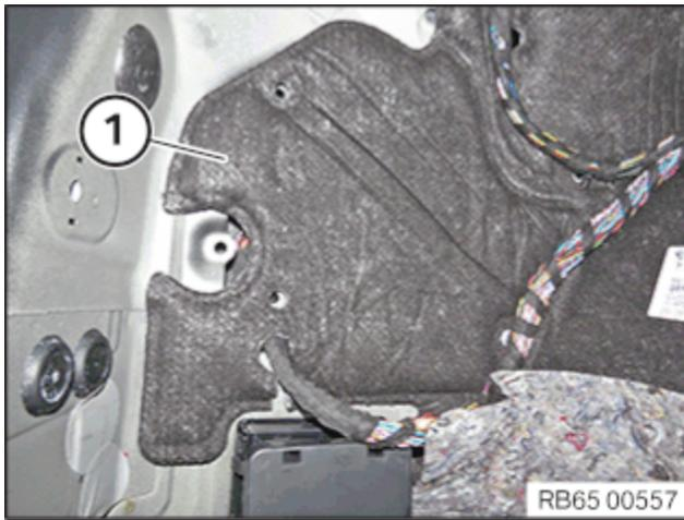
Lay insulating mat (1) correctly.
