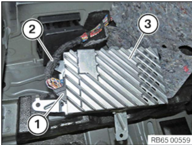
Unlock and disconnect the connector (1).
