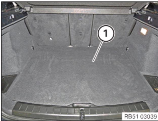
Attach luggage compartment floor trim panel (1) at front in hooks and lay down at rear.
