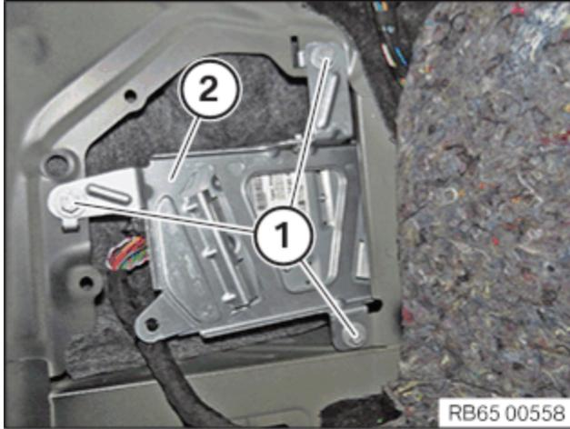
Correctly position amplifier with holder (2).
