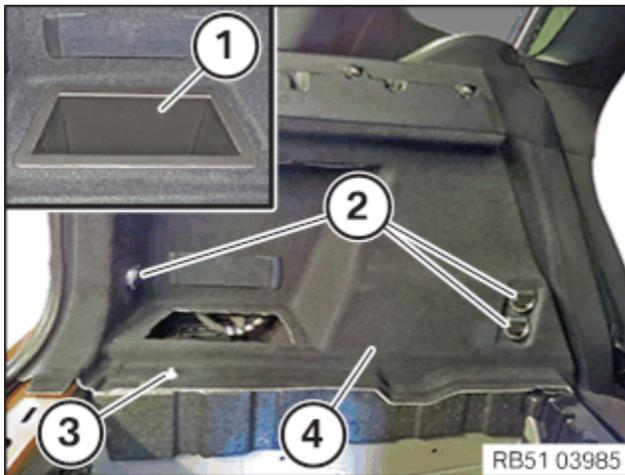
Lift out storage compartment (1) upwards.
