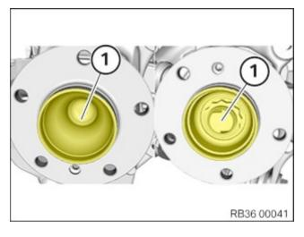
• Apply a thin layer of grease to the front and rear wheel hubs (1) to protect against corrosion.
