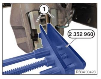
• Press back the brake piston up to the limit position.
