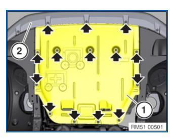
Feed in underbody protection (1) under bumper panel (2) and position.
