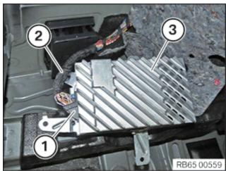
Position amplifier with holder (3). Connect and lock the connector (1). Clip in cable clip (2).
