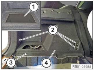
Lift out storage compartment (1) upwards.
