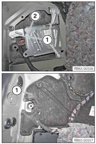
Correctly position amplifier with holder (2).
