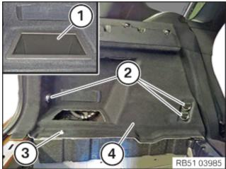
Insert the trim panel (4) and tighten the pin (3).
