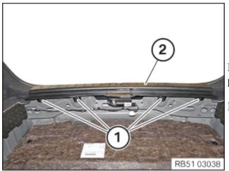
Release expanding rivets (1) from tail panel trim (2).
