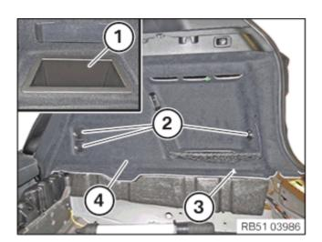
Lift out storage compartment (1) upwards.
