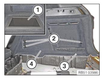
Insert the trim panel (4) and in this process, connect the plug connections.
