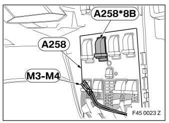
Connect branches **M3-M4** as follows to plug **A258\*8B**, SW 54-pin socket housing, on BDC **A258**:
