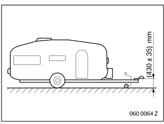
Figure **3**Installation height for the towing ball coupling.
