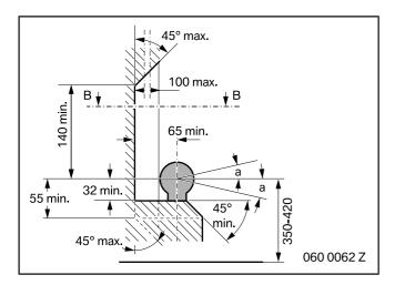
Figure **1**Space for coupling ball, side view.
