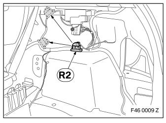
The installation site of bus interface **R2** may vary. When connecting .branches **A6-A7**, use the ISTA/AIR documentation to ensure that bus interface **R2** is used. ◀
