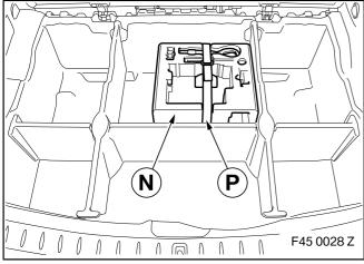
Insert oddments tray  ${\bf N}$  into the spare wheel trough and lash tightly in lace using Velcro strip  ${\bf P}$ .
