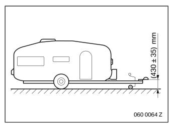
Installation height for the towing ball coupling.
