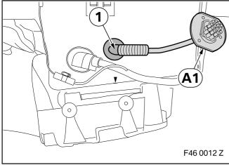
Insert grommet (1) into the hole so it is waterproof. Route cable branch **A1** outside the car.
