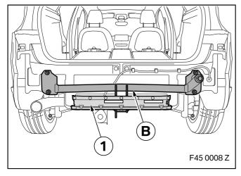
Fit the support (1) using the existing fastening material to trailer tow hitch **B**.
