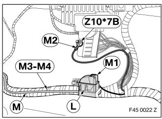
Connect bus interface retrofit wiring harness  ${\bf M}$  as follows:
