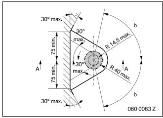
Figure **2**Space for coupling ball, plan view.
