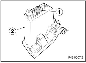
Modify the support (1) of the storage compartment (2) for the cable bushing as required.
