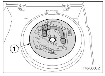
Remove the ball head. Store the ball head in the spare wheel trough (1).
