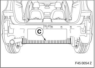
Fit heat insulation **C** using existing fastening material.
