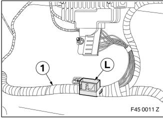
Secure bus interface **L** using insulating tape to the standard wiring harness (1).
