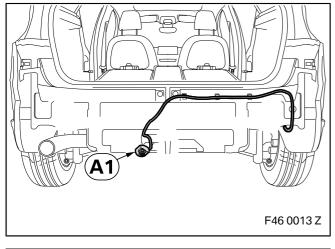
Route the cable branch **A1** outside the car to the location of the trailer tow hitch.
