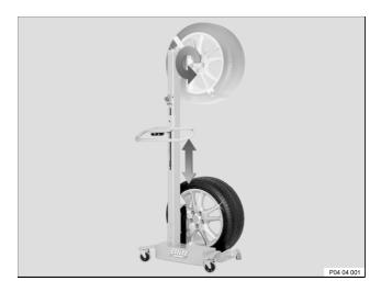
• In vehicles with M Carbon ceramic brake: The wheel assembly jack must be used to remove the wheel (see workshop equipment).
