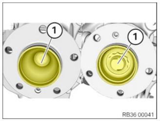
• Apply a thin layer of grease to the front and rear wheel hubs (1) to protect against corrosion.
