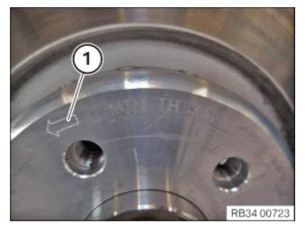
If an arrow 1 is engraved on the brake discs, then it must show the direction of travel!
