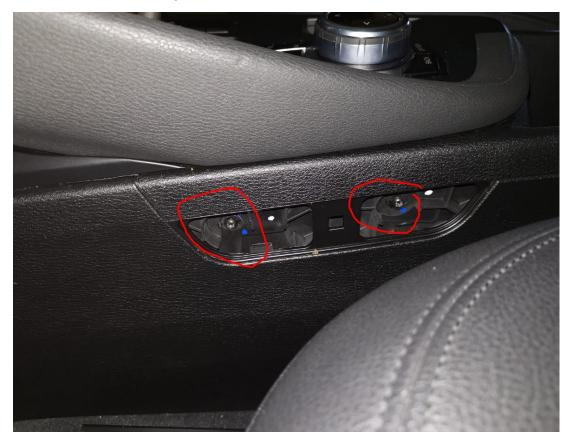
Remove plastic liner in the centre storage and expose 1 hex screw.
